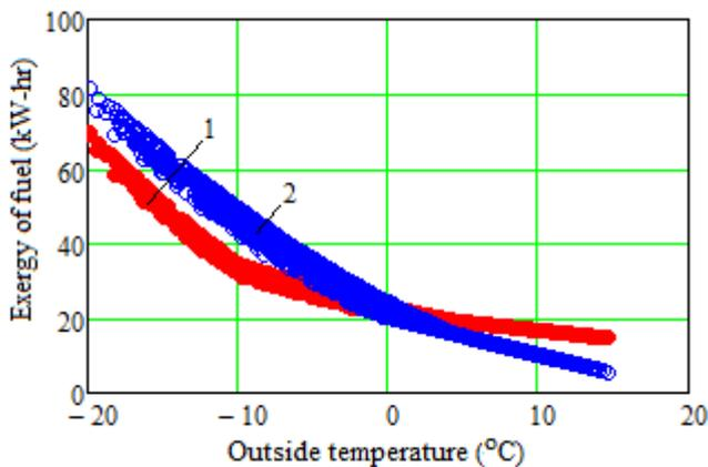
Figure 3. Exergy of fuel expended to provide the ventilation air versus outside temperature for the control volume 2: 1 - with heat recovery; 2 - without heat recovery
