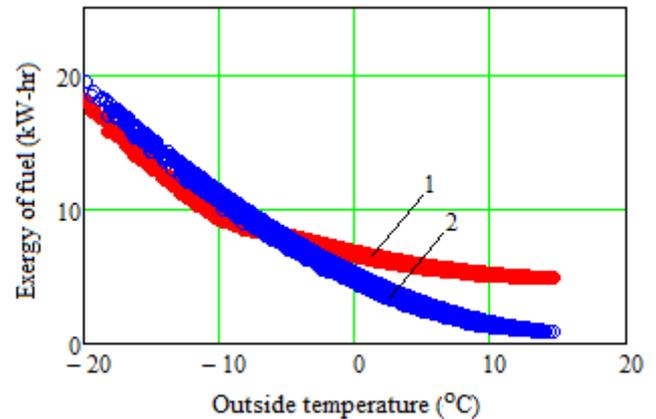
Figure 2. Exergy of fuel expended to provide the ventilation air versus outside temperature for the control volume 1: 1 - with heat recovery; 2 - without heat recovery
