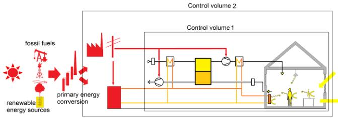
Figure 1. Energy supply chain for space heating in a buildings from primary energy transformation to final energy, including all intermediate steps up to the supply of the heating demand
