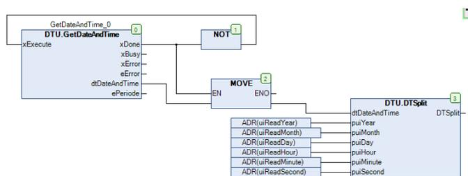
Figure 2. The program for reading the date and the time from the PLC
