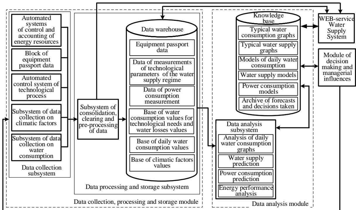
Figure 2. The architecture of operational control of energy efficiency modes of water supply facilities
