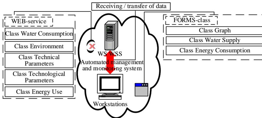
Figure 1. The architecture of operational control of energy efficiency modes of water supply facilities
