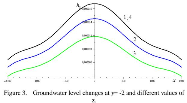
Figure 3. Groundwater level changes at  $y=-2$  and different values of  $z$ .
