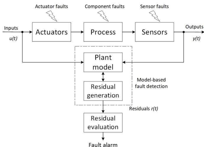
Figure 1. Model-based fault detection scheme
