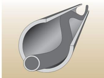
Figure. 1 Contact of the bent part of the drillstring with the cylindrical wall of the well
