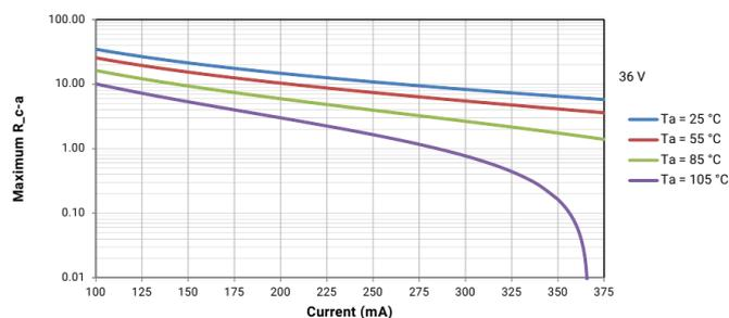
Figure 4. Maximum thermal resistance between contact and air
