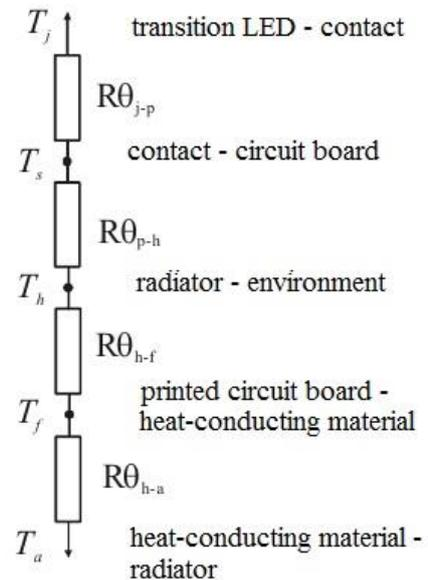
Figure 3. Equivalent circuit for LED CXA1507
