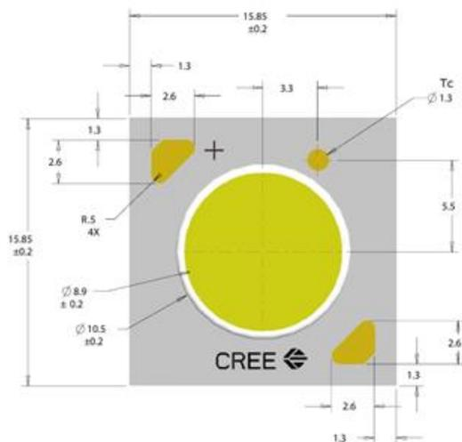
Figure 1. Mechanical characteristics of the CXA1507 LED
