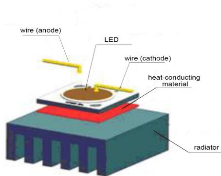
Figure 2. Installation of CXA1507 LED on the radiator
