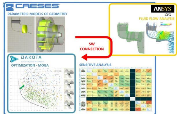
Figure 3. Workflow for automatic runner shape optimization
