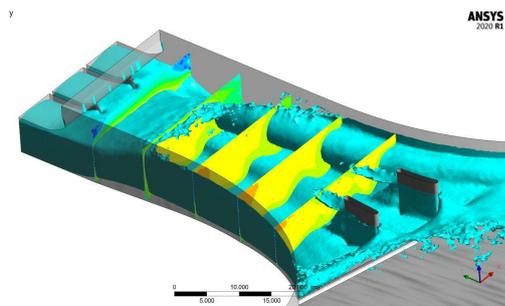
Figure 2. Example of low head HPP intake simulation
