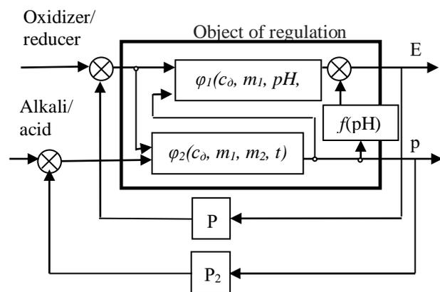
Figure 2. Structural scheme of two-channel system of regulating the dosage of reagents:  $P_1$  - regulator Eh;  $P_2$  - regulator pH;  $\varphi_1$  - function of transforming redox process;  $\varphi_2$  - function of transformation of process of acidification;  $f(pH)$  - dependence Eh on pH;  $c_o$  - concentration of admixtures;  $m_1$  - mass of added reducer;  $m_2$  - mass of added acid;  $t$  - time
