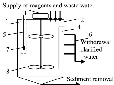
Figure 3. The scheme of the mixer-reactor of periodic action with mechanical stirring and with the function of settling: 1 - electric motor with gearbox; 2 - the housing of the mixer reactor; 3 - perforated protective tube; 4 - vertical plates; 5 - rods for fastening pH and Eh converters; 6 - pipelines for drainage of clarified water; 7 - pH and Eh converters; 8 - the blades of the mixer
