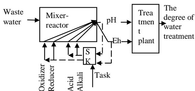
Figure 1. — Structural scheme of wastewater treatment with regulation of pH and Eh with the introduction of various reagents (SK - control system)
