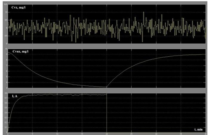
Figure 3. Change in Cvx inlet concentration, Cvux outlet concentration, and current I between plates
