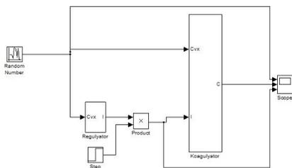
Figure 1. Simulation model of electrocoagulator
