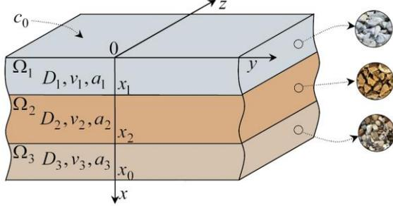
Figure 1. Three-layered filter in which particles of pollution migrate
